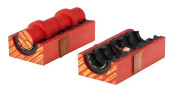
EMC modules with contact tips and tapes (made from electrolytic copper) form a conductive connection between cable shield and frame.
